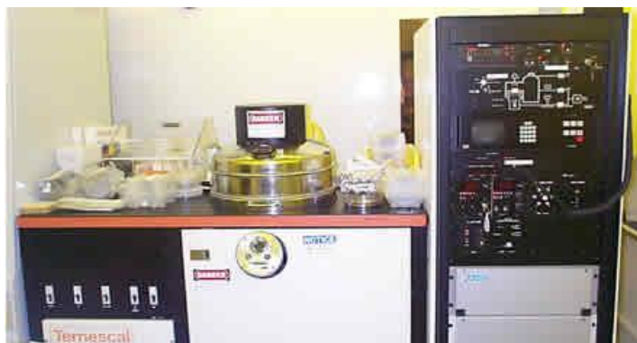
Figure 2.8: BJD 1800 E-beam evaporation system for metal deposition[44]
